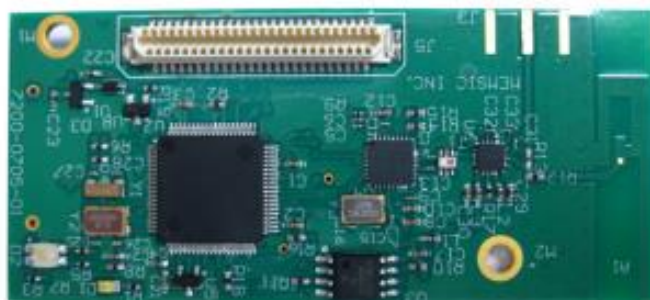
Figura 15 – Nó sensor LPR2400 (Lotus Mote) (fonte: MEMSIC, 20--)
